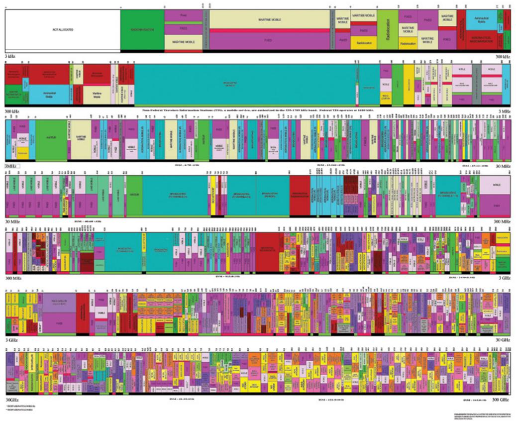
Figure 1. A frequency spectrum chart shows the dense packing of RF and microwave allocations.
