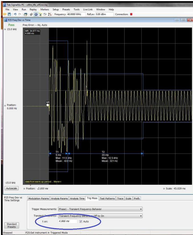
Figure 20. Transient Frequency Behavior measurement control.
