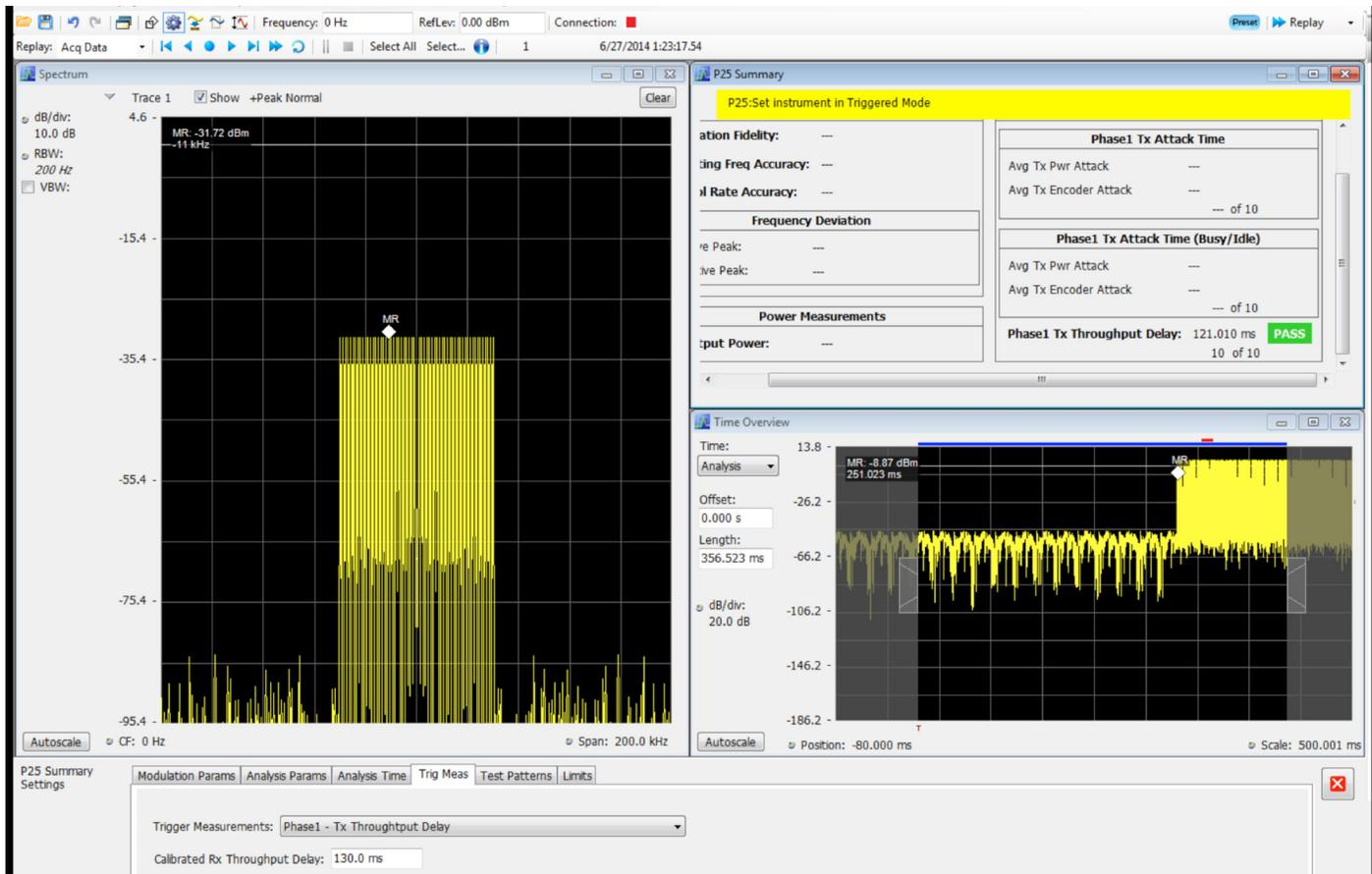
Figure 18. Transmitter throughput delay results cross related across multiple displays.
