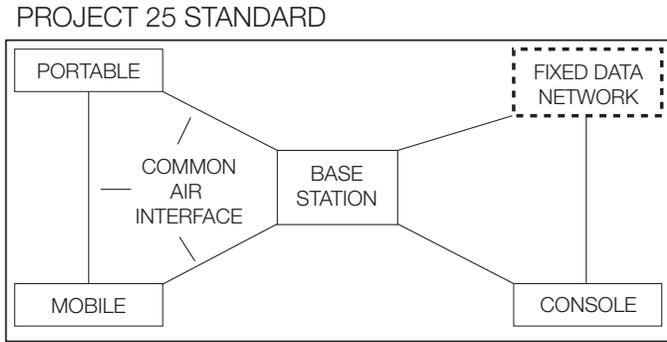
Figure 1. P25 Common Air Interface.
