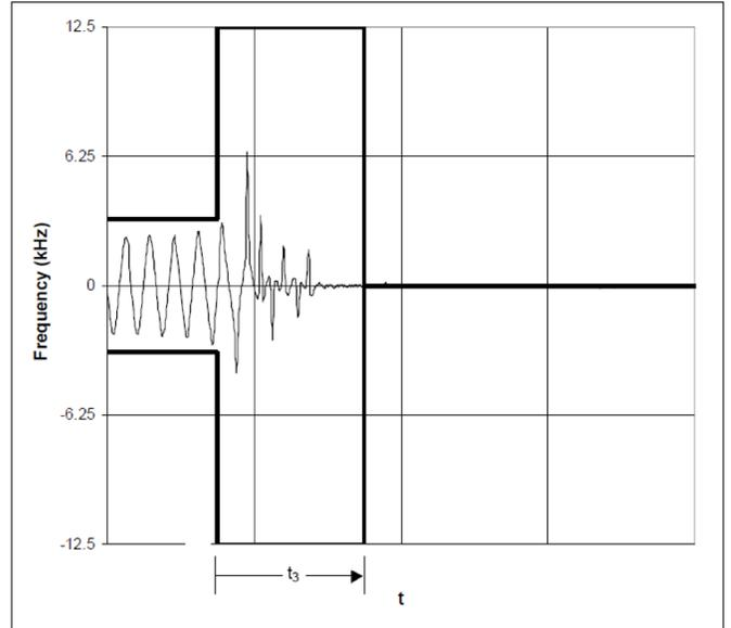
Figure 19.2. Turn-off transient behavior and mean frequency limits.
