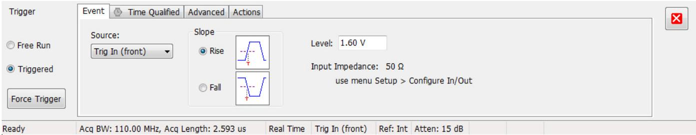
Figure 15. Operating Tektronix RSA5000 in triggered mode.
