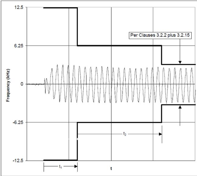
Figure 19.1. Turn-on transient behavior and mean frequency limits.
