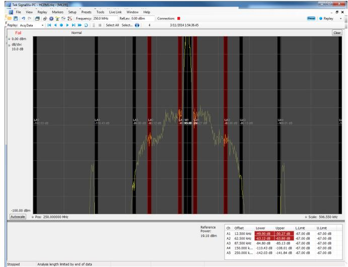
Figure 6.2. Adjacent Channel Power Ratio measurement failing.
