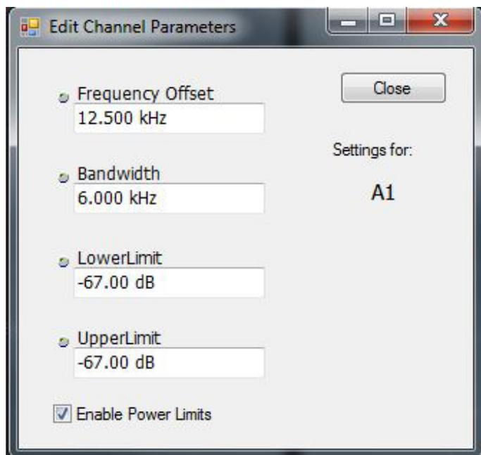
Figure 7 shows a screenshot of the MCPR settings control panel. Once the user selects a row in the adjacent channels' table, he can choose to delete or edit that row. In particular the user can edit the limits.
