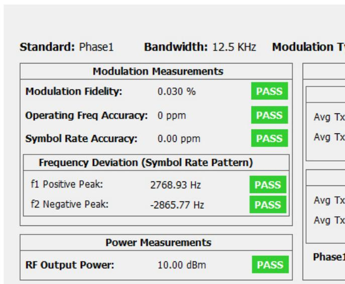
Figure 13. P25 Summary provides for Symbol Rate Accuracy and Frequency Deviation measurements of a symbol rate test pattern.
