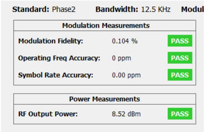
Figure 8. P25 Summary for scalar measurements with Pass/Fail information.
