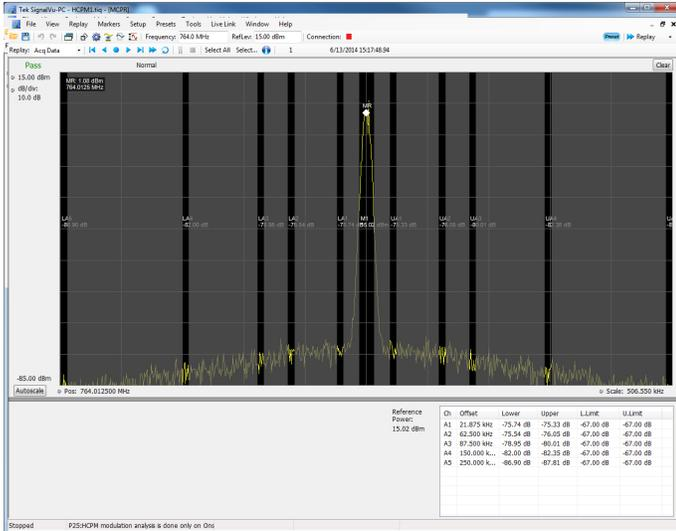
Figure 6.1. Adjacent Channel Power Ratio measurement passing.
