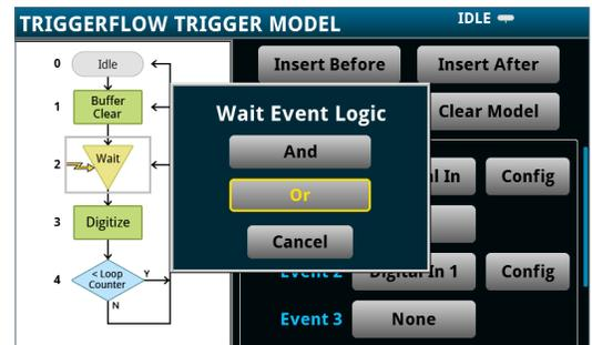
TriggerFlow enables logic trigger
