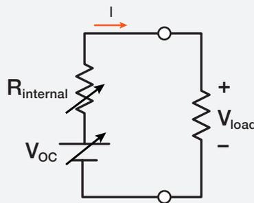
$$V_{load} = V_{OC} - (I \times R_{internal})$$
