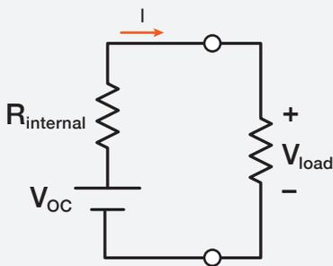
$$V_{load} = V_{OC} - (I \times R_{internal})$$
