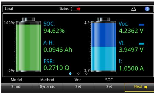
Use a battery simulator to monitor State-of-Charge, Amp-Hours, equivalent series resistance, open circuit voltage, terminal voltage, and load current.
