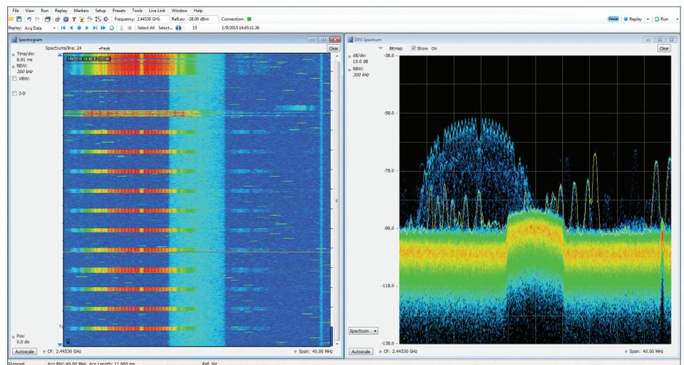
**Figure 4.** An RTSA provides complete domain correlation allowing information in the spectrogram on the left to be directly correlated with other measurements.
