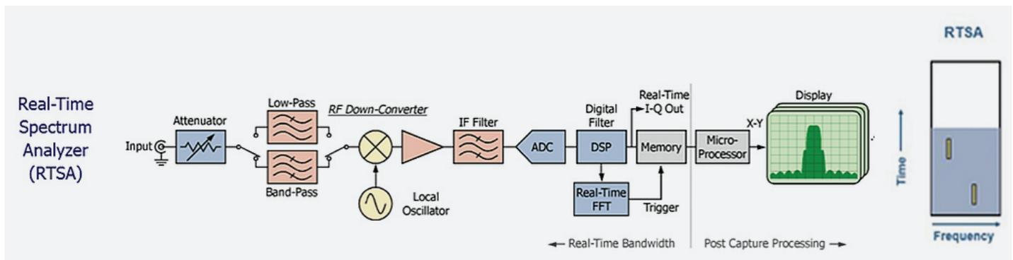
**Figure 2.** This is the block diagram of a basic real-time spectrum analyzer.
