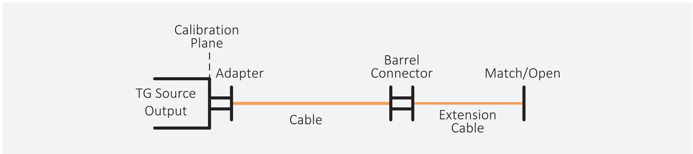
FIGURE 9. Typical Distance to Fault Measurement Setup.
