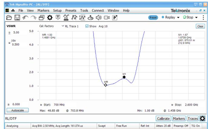
FIGURE 3. VSWR vs. Frequency of a bandpass filter.
