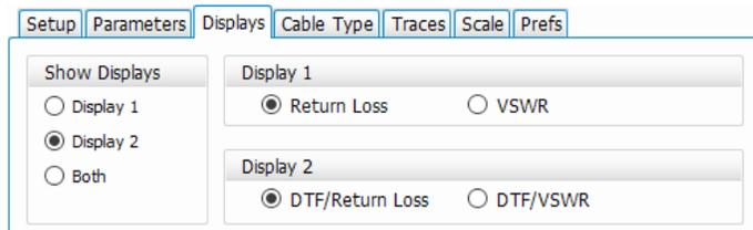
FIGURE 5. DTF setup in SignalVu-PC.
