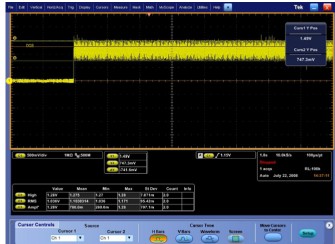
Figure 2 Output with high temperature (~120 degrees F) testing as measured using a DPO7254 Oscilloscope
