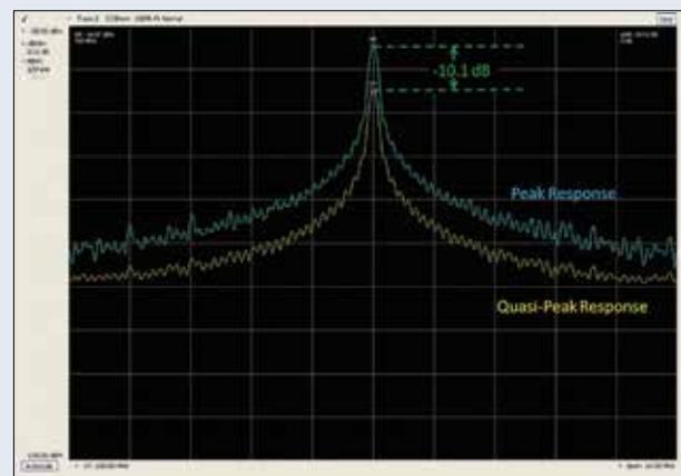
**Figure 3.** Comparison of peak detection and quasi-peak detection.
