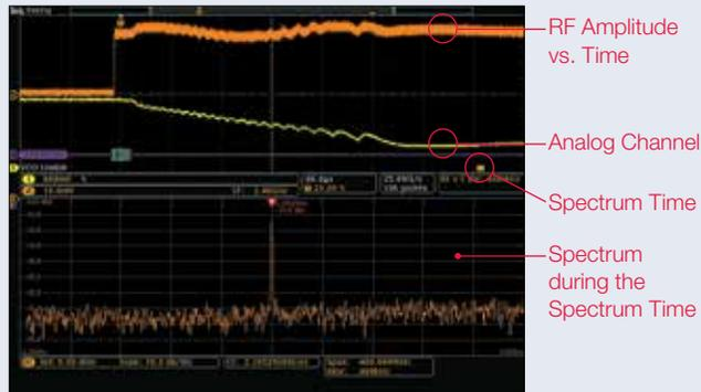
**Figure 9.** An MDO4000 Series oscilloscope provides a time-correlated view of an oscillator start-up.
