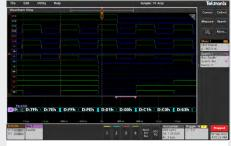
Optional 16-channel MSO to trigger, capture, measure and decode digital signals on embedded designs.
