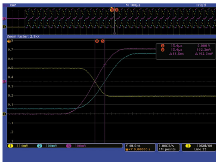
Figure 12b. Measuring the delay in the Pb signal due to an additional length of cable or processing time.
