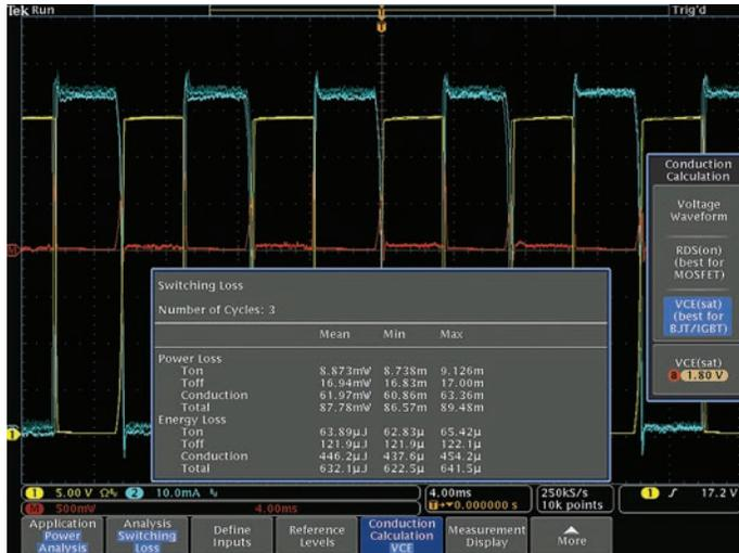
Figure 13. Switching Loss Measurements on an IGBT.
