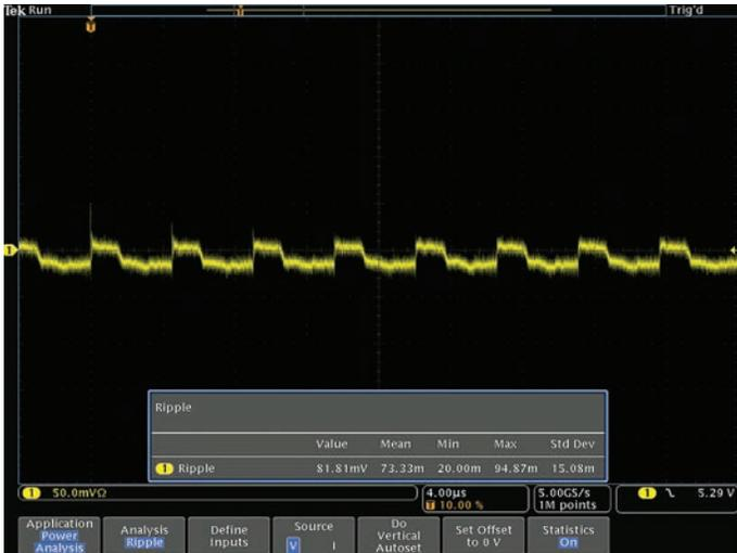
Figure 17. Ripple Measurements.
