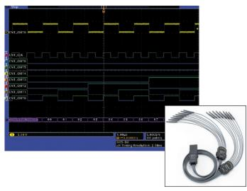
Figure 4. Probe color coding matches waveform color coding, making it easier to see which signals corresponds to which test point.
