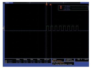
Figure 9. TTL Burst Signal.
