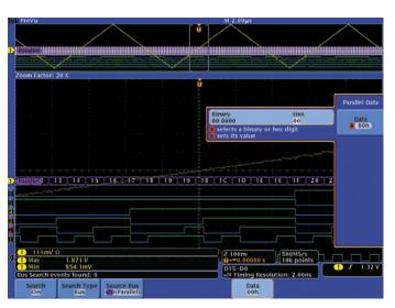
Figure 25. Wave Inspector search finds no 00 hex values at test signal valleys.
