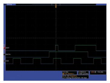
Figure 19. D-Flip-Flop Q output error.
