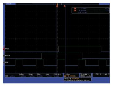
Figure 16. D-Flip-Flop operation looks normal based on one acquisition.
