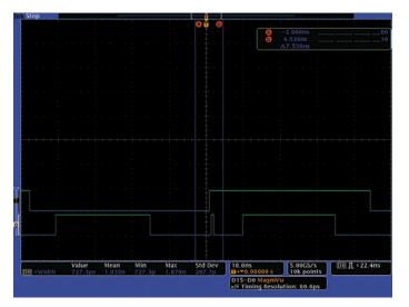
$\textbf{Figure 13.} \ \, \textbf{MSO} \ \, \textbf{triggered on 727.3 ps glitch on the bottom LVPECL signal.}$
