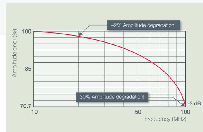
Bandwidth is defined as the frequency at which a sine-wave input signal is attenuated to 70.7% of its true amplitude (the -3 dB or 'half-power' point, shown here for a 100 MHz scope).
