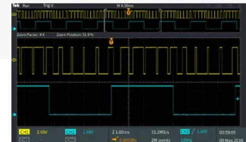
Since an oscilloscope can store only a limited number of samples, the waveform duration (time) will be inversely proportional to the oscilloscope's sample rate. **Time Interval = Record Length / Sample Rate**
