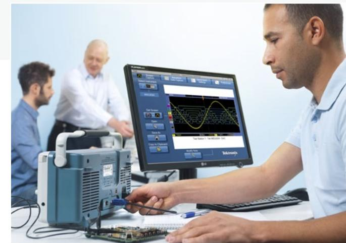
Standard interfaces can include USB, Ethernet, GPIB, Wi-Fi, or RS-232. USB is currently the most common interface, since it is included on most computers and is convenient to use. Ethernet is electrically robust and allows for remote connection over the Internet.
