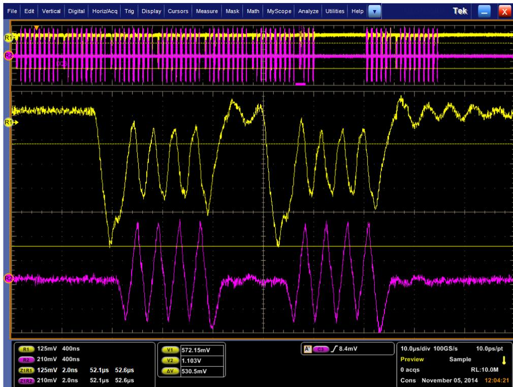
Figure 14- DDR4 Memory Lab Measurements with DDR4 Interposer
