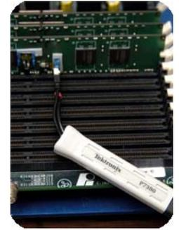
FB-DIMM signal measurement using P7313 probe
