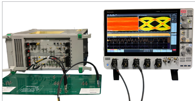
Figure 2: A BERT (left) is used to drive PRBS test signals through PCB traces of 24in length and a pair of 1-meter SMA cables. The 7 Series DPO with Advanced Jitter Analysis software (option DJA) and Signal Integrity Modeling software (option SIM) is used to measure the resulting signal.
