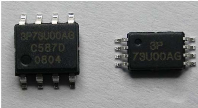
First in the world, the PulseCore 3P73U00AG ICs provides SSC for a variety of USB 2.0 ASIC input clock frequencies (12MHz, 15MHz, 24MHz, 25MHz, 30MHz, 48MHz, etc). The SSC function maintains USB 2.0 compliance and attenuates the 480MHz fundamental USB 2.0 radiated frequency by 4dB.
