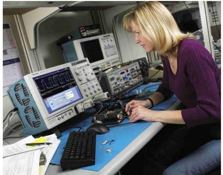
Tektronix DPO7000 with TDSUSB2 automated USB compliance software
