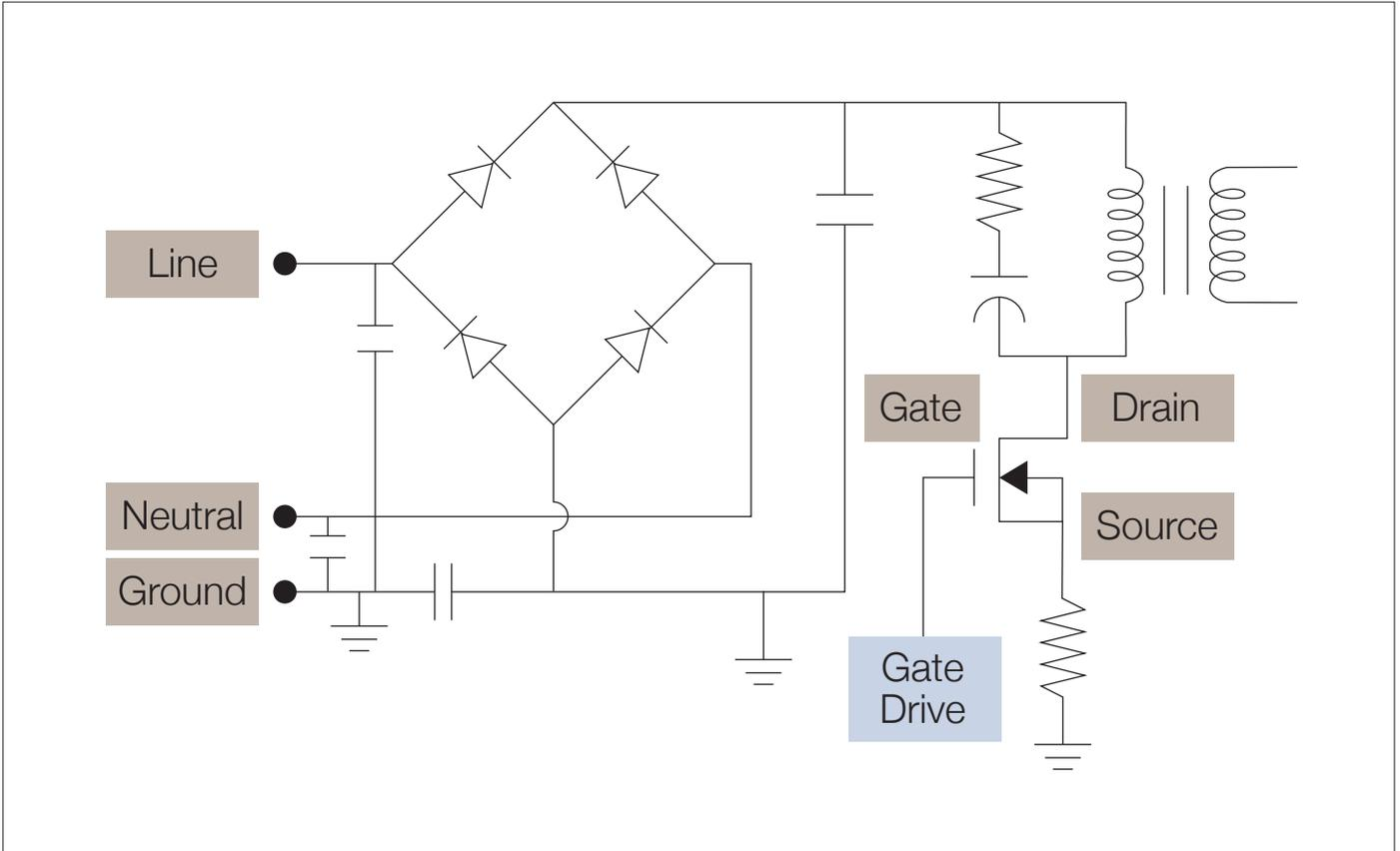
Figure 1. Simplified switch mode power supply switching circuit.
