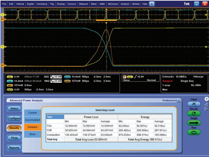
Figure 5. DPOPWR automated switching loss measurement.
