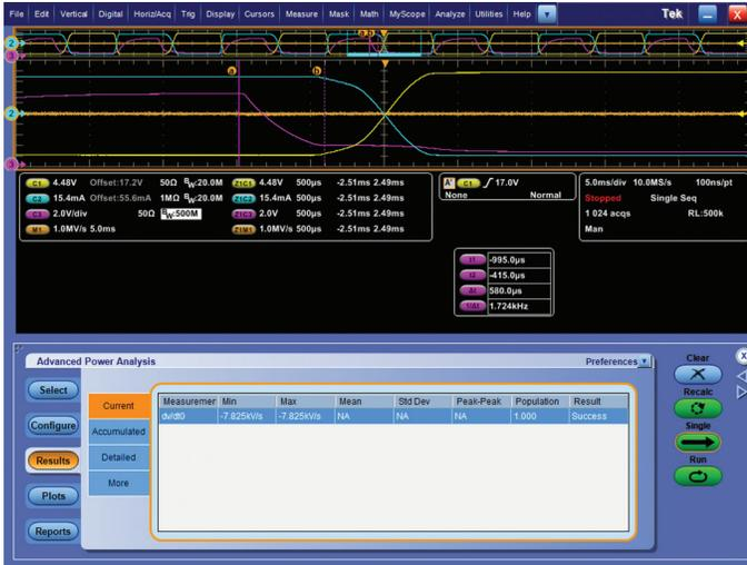
Figure 7. Automated slew rate measurement on MOSFET gate.
