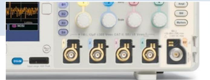
A mixed domain oscilloscope not only offers analog and digital channels, like an MSO, but also includes a dedicated RF input channel that behaves like a spectrum analyzer.
