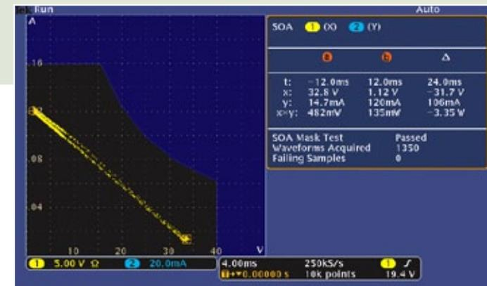
Is your SMPS switching device operating within safe limits?
