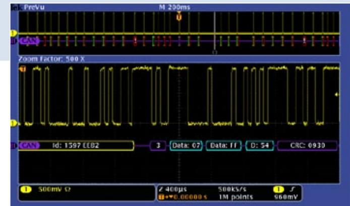
Oscilloscopes with record lengths in the millions of points can show thousands of screens worth of signal activity, essential for examining complex waveforms. Placing **marks** on the waveform assists in latency measurements on a CAN bus, for example.
