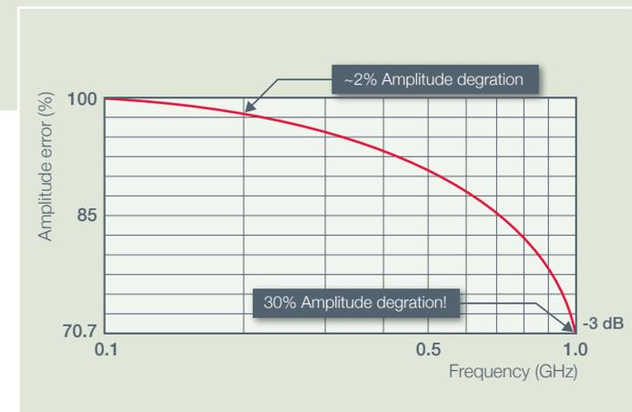
Bandwidth is defined as the frequency at which a sine-wave input signal is attenuated to 70.7% of its true amplitude (the -3 dB or 'half-power' point, shown here for a 1 GHz scope).
