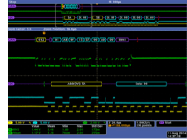
Figure 3. CAN and I2C decoding helped to speed up debug.
