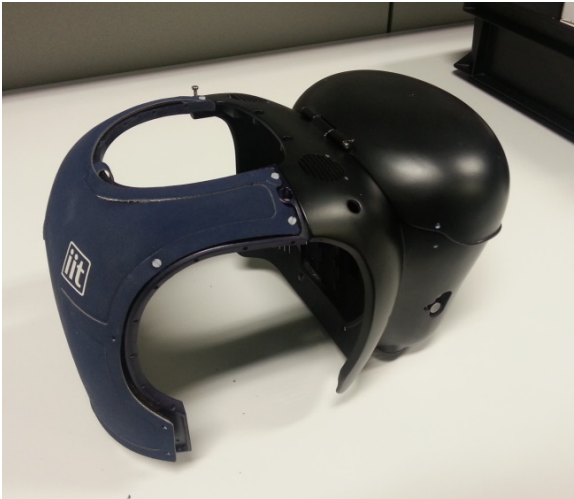
The new battery backpack contains a 36V-9.3Ah Li-On power source, enough to power the iCub for several hours of operation.
