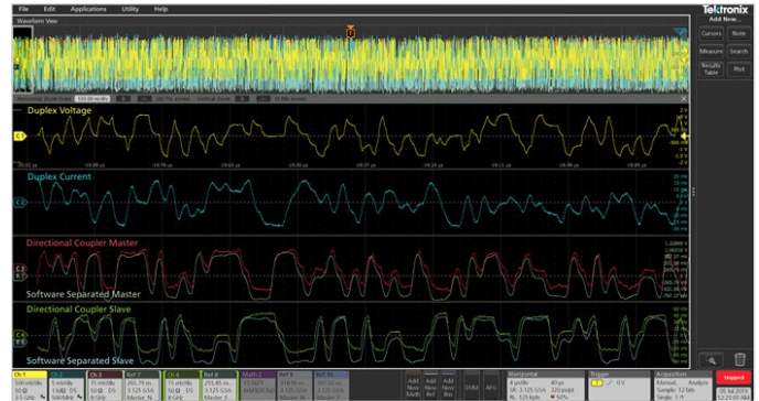
Test results comparing Tektronix Signal Separation and the directional coupler methods.
