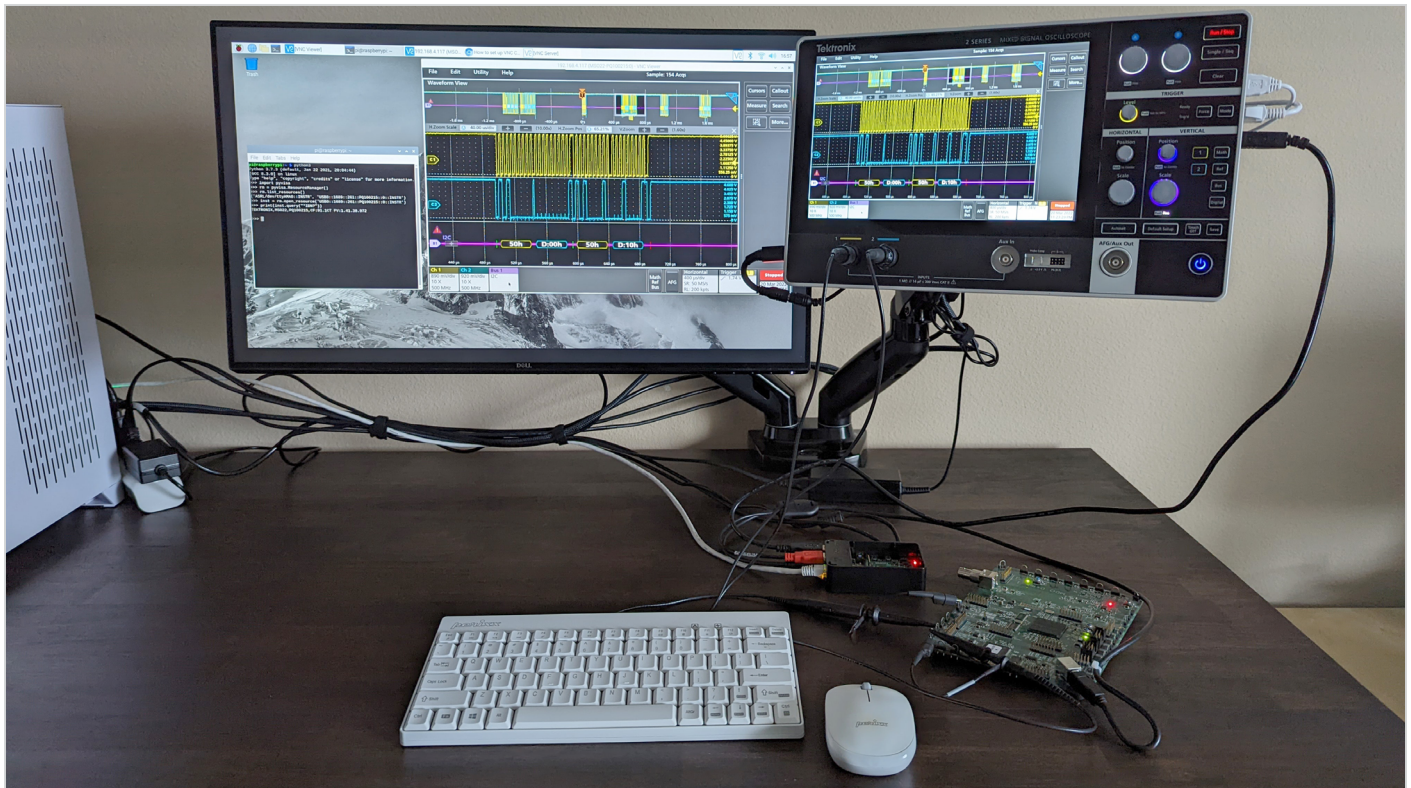
Figure 1: A quick setup for the Tektronix 2 Series MSO Mixed Signal Oscilloscope and a Raspberry Pi.
