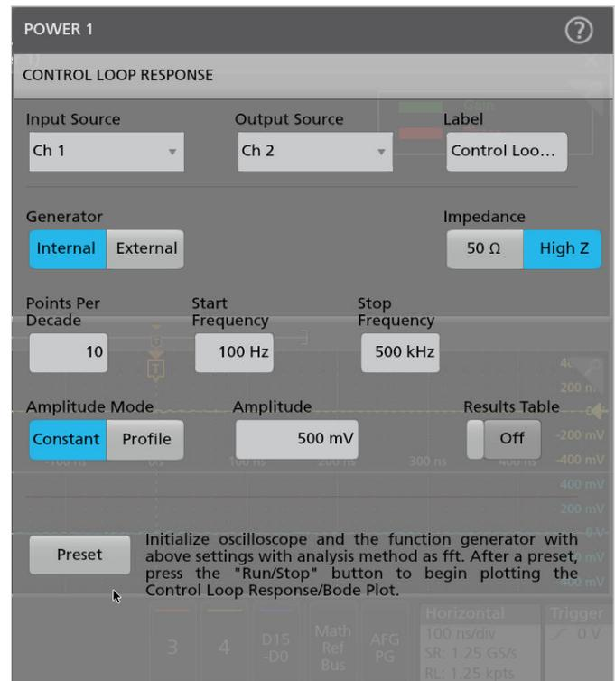
Figure 5: Bode plots configuration using internal AFG.
