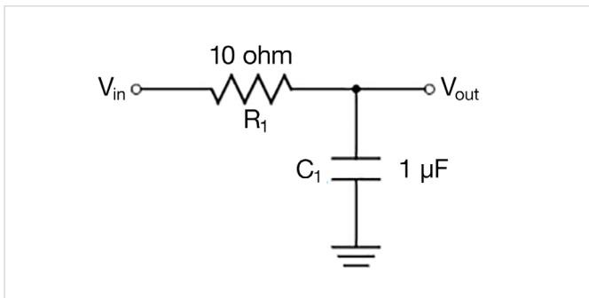
Figure 3: Simple passive low pass filter with RC network.
