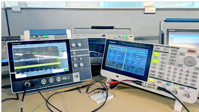
Figure 8: Using the AFG31000 with 2 Series MSO to generate bode plots.
