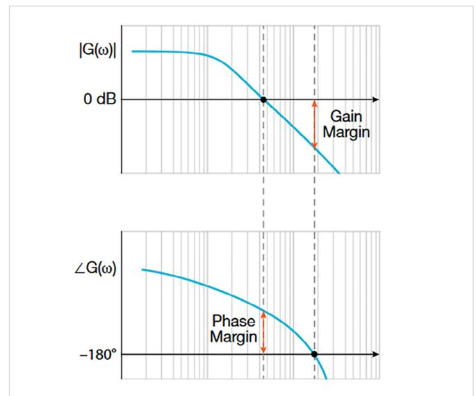
Figure 2: Gain and phase margin.
