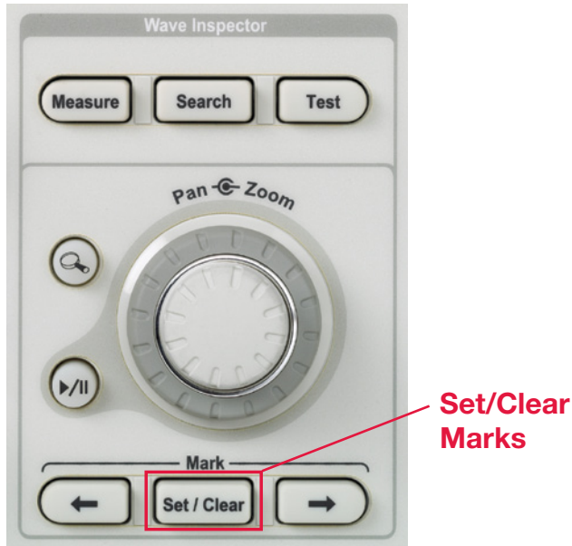
Figure 2B. Dedicated front-panel controls for setting/clearing marks and navigating between them.
