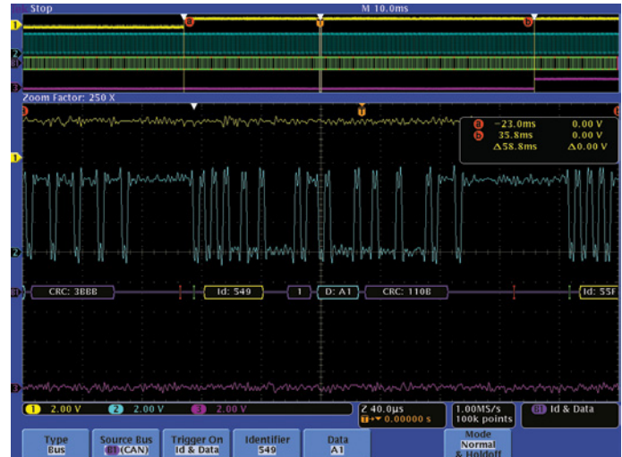
Figure 3. Placing marks on the waveform to assist in latency measurements on a CAN bus.
