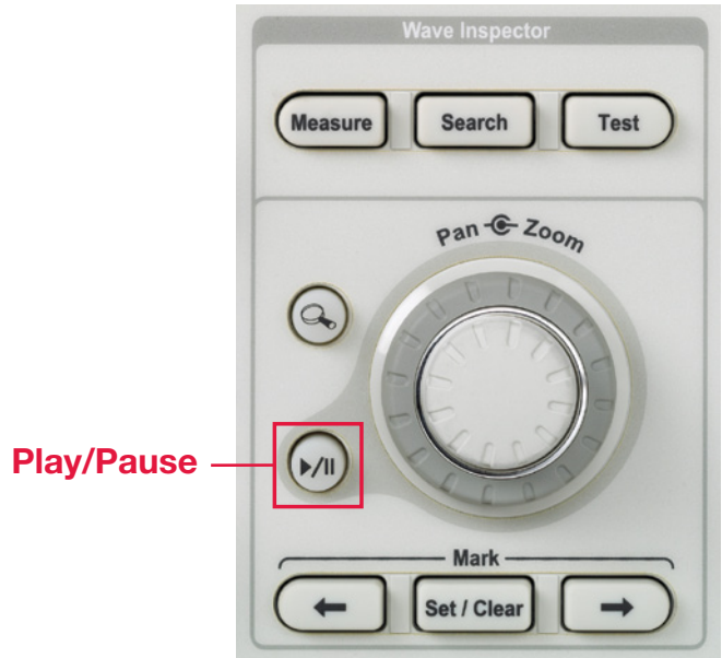
Figure 2A. Dedicated front-panel control for automated waveform playback.
