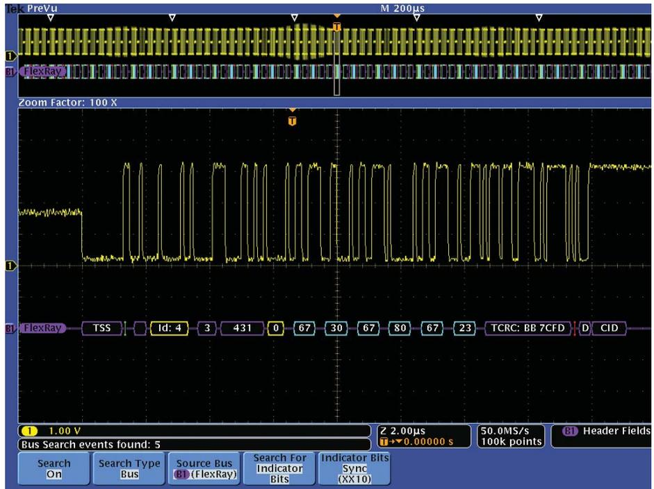
Figure 26. Triggering on Frame ID and Cycle Count, Searching through acquired data for Startup Frames.
