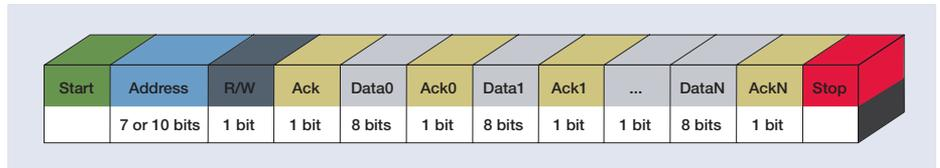
Figure 4. I<sup>2</sup>C message structure.
