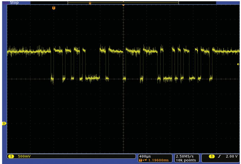
Figure 2. One message acquired from a CAN bus.
