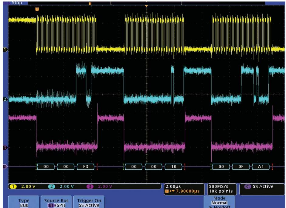
Figure 13. Correct synthesizer configuration messages.
