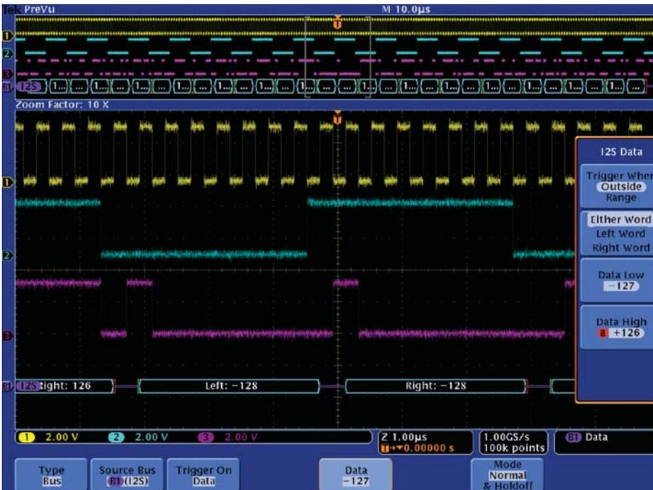
Figure 32. Triggering outside a range of values on an I<sup>2</sup>S bus.
