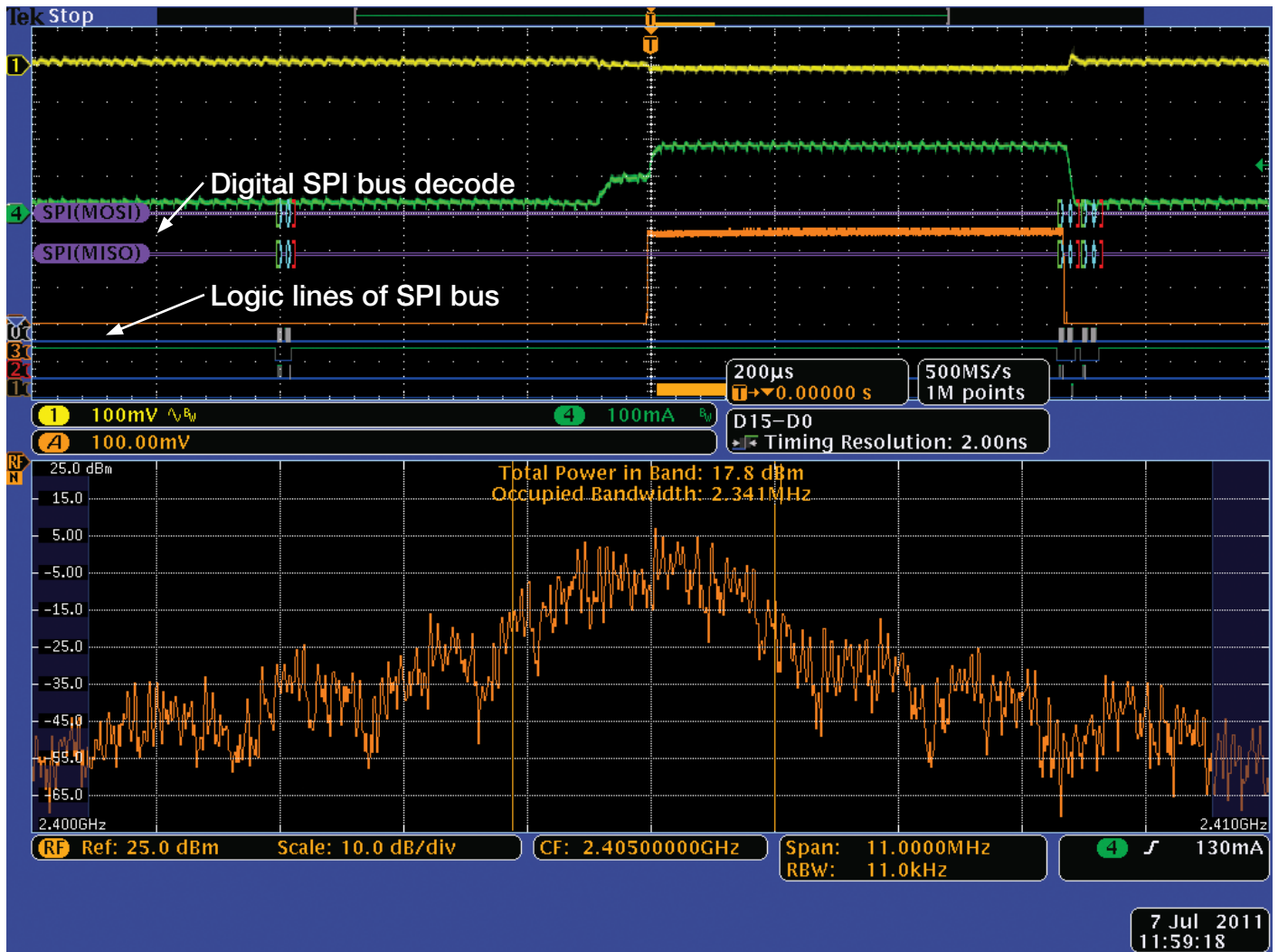
Figure 7. Packet decode of SPI Digital signals (SPI - MOSI and MISO) added to display.
