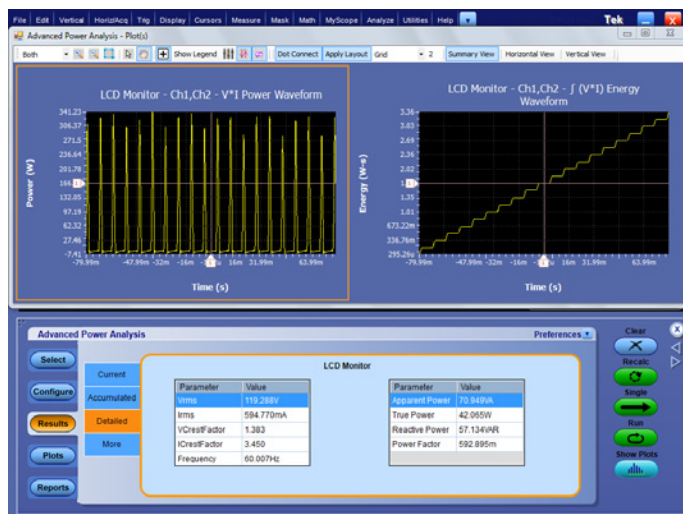
Figure 9. Power Quality Measurements on an LCD computer monitor, while it is on.
