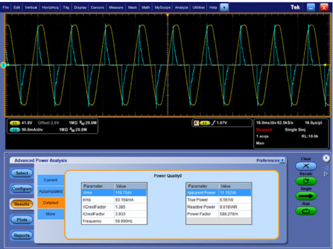
Figure 14. Power Quality Measurements on a cell phone charger while the phone is charging.
