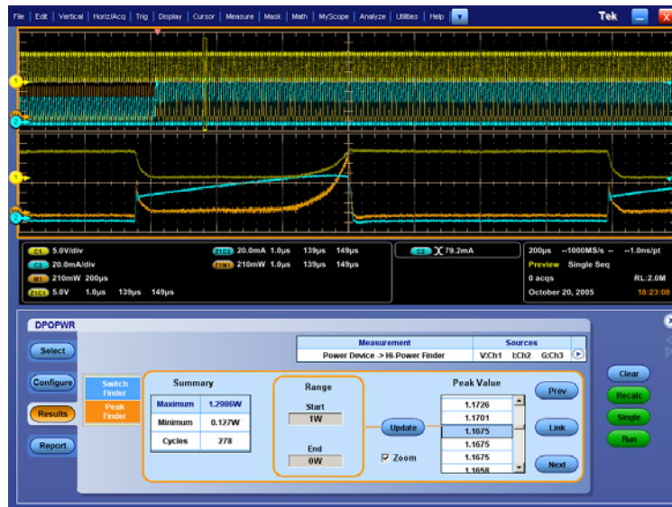
Figure 7: Using HiPower Finder and the oscilloscope's zoom feature to analyze the power waveform at the switching device during load change.
