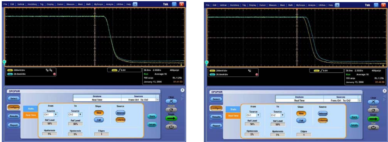
Figure 5: (a) Differences in propagation delay for the measured voltage and current signal. (b) The difference in propagation delay is eliminated after using the Auto Deskew operation that is a part of the DPOPWR power analysis software.
