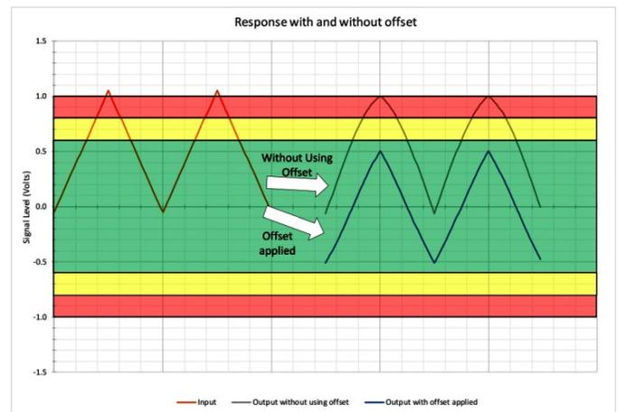
The green, yellow, and red areas correspond to  $\pm 60\%$  range,  $\pm 80\%$  range, and  $\pm 100\%$  range, respectively. TIVH DC Gain accuracy is most accurate within the green range with a  $\pm 3\%$  specification and falls to  $-7\%$  at the extreme 100% edge.
