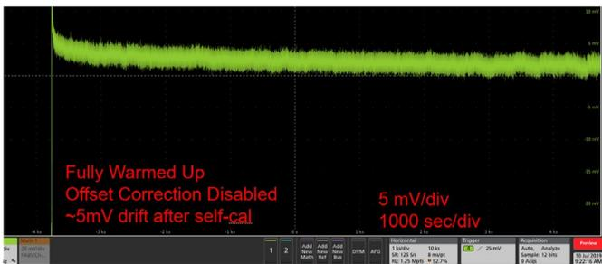
**NOTE:** All numbers in this post are “input referred” meaning they were taken without any tip attached. The tip attenuation and Range setting will multiply the error. For example, 100 mV of drift will show as 5 V of drift with a 50X tip attached in 1X range setting.
