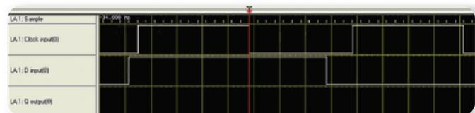
▶ **Figure 15.** Logic analyzer triggering on a flip-flop error.
