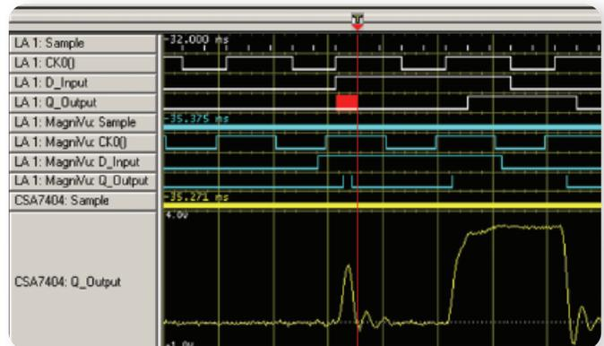
▶ **Figure 9.** Logic analyzer triggering on and capturing a flip-flop Q output glitch.
