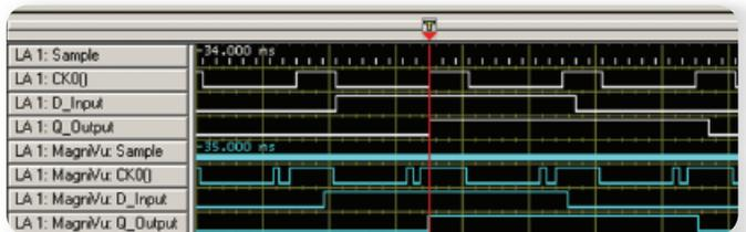
► Figure 3. Flip-flop deep timing 2 ns resolution waveforms and MagniVu 125 ps high-resolution timing waveforms.
