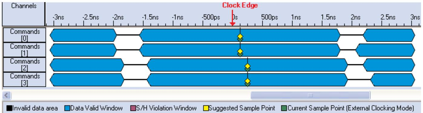
**Figure 17.** Logic analyzer AutoDeskew analysis shows the suggested sample point position with yellow diamonds. The green diamonds show the current sample point position, which has been set equal to the suggested position.
