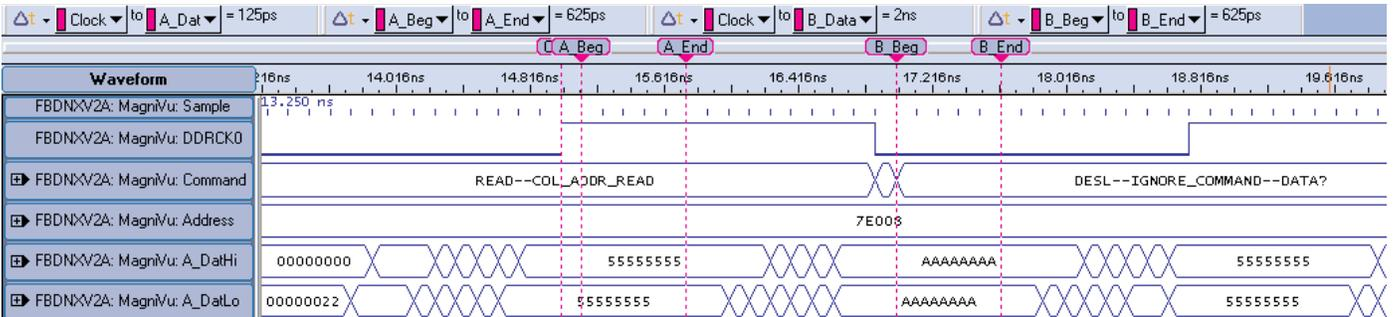
**Figure 34.** MagniVu high-resolution timing measures the read data valid windows to set the logic analyzer sample point position. The DDR2 SDRAM 64-bit read data is an alternating pattern of 5555,5555,5555,5555 hex and AAAA,AAAA,AAAA,AAAA hex.
