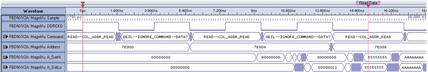
**Figure 33.** Trigger on the first Read command after the Activate command. Count the four Read Latency (RL) clock edges to find the first read data cycle shown with a Read Data marker. The DDR2 SDRAM 64-bit read data is an alternating pattern of 5555,5555,5555,5555 hex and AAAA,AAAA,AAAA,AAAA hex.
