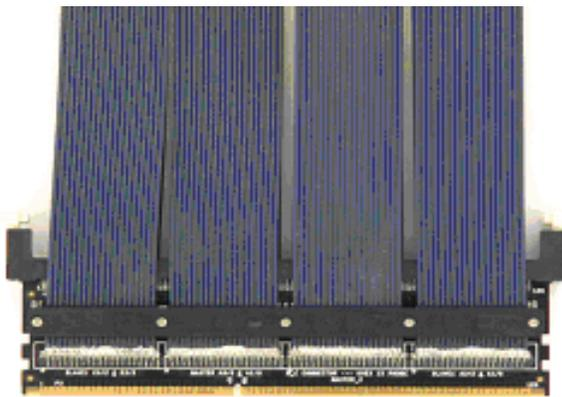
Figure 2. DIMM Interposers
