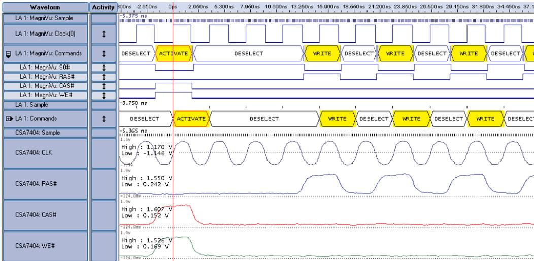
**Figure 20.** The logic analyzer iCapture probe provides simultaneous probing for three different types of SDRAM clock and commands measurements. The top waveforms are MagniVu 125 ps high-resolution timing. The middle Commands busform is state acquisition. The bottom four waveforms are the CLK, RAS#, CAS# and WE# from the oscilloscope using the iView interface.
