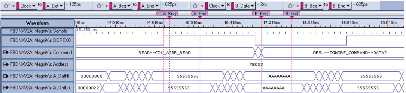
**Figure 34.** MagniVu high-resolution timing measures the read data valid windows to set the logic analyzer sample point position. The DDR2 SDRAM 64-bit read data is an alternating pattern of 5555,5555,5555,5555 hex and AAAA,AAAA,AAAA,AAAA hex.
