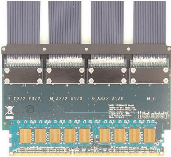
**Figure 31.** Nexus DDR3 NEXVu DIMM designed to JEDEC standards with logic analyzer probe points. This provides unmatched signal fidelity and allows the capture of the actual eye patterns as seen by the memory components.
