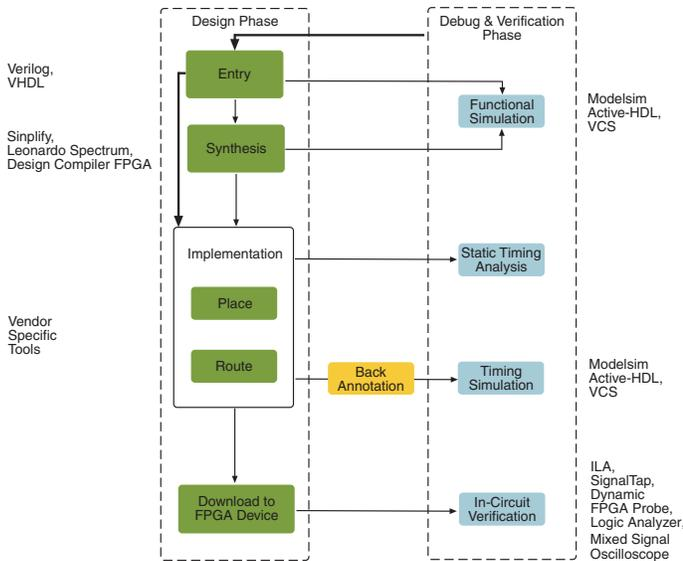
Figure 1. FPGA Design Flow.
