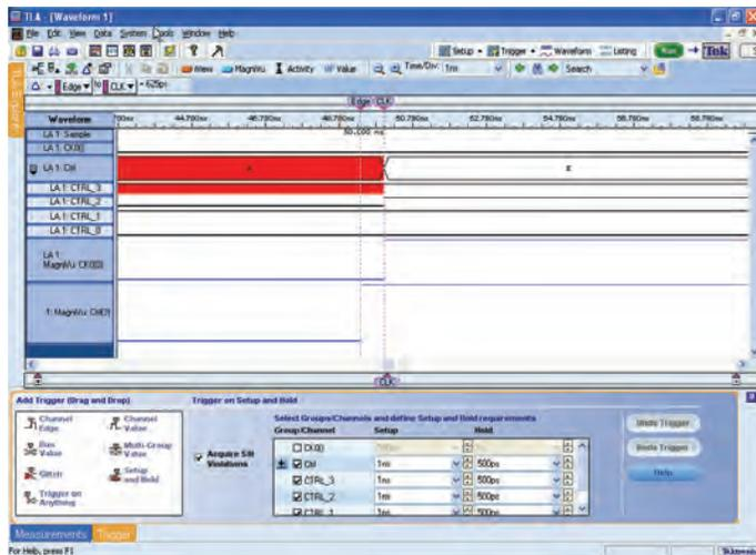
Figure 20. MagniVu provides measurements and clues about a violation.
