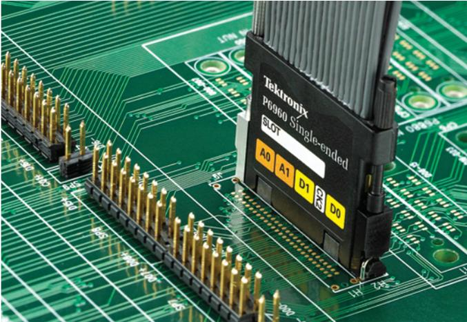
Figure 2. D-Max connectorless logic analyzer probe.
