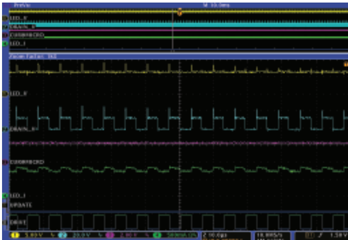
Figure 3.6. LED operation with current hysteresis value of 8 magnified.
