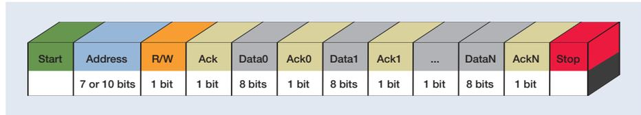
Figure 5.1. I<sup>2</sup>C message structure.
