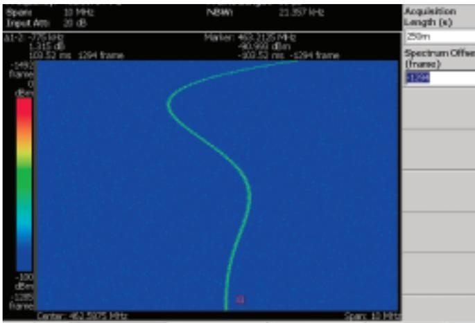
Figure 8.3. Spectrogram showing oscillator turn-on settling characteristic enables measurement frequency variance over time.
