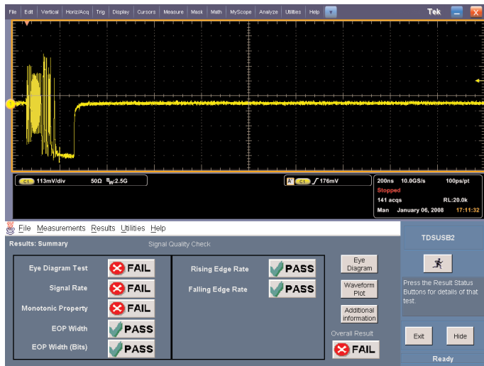
Figure 1.4. Waveform and signal quality report for the extended 10 meter USB cable in high speed operation.
