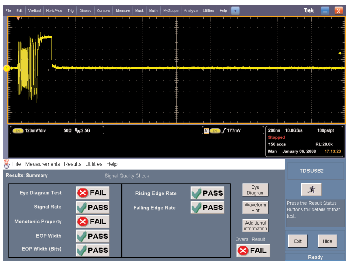
Figure 1.6. Waveform and signal quality report for the extended 7.5 meter USB cable in high speed operation.
