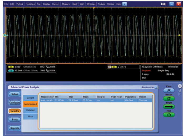
Figure 11. Inductance as measured by the DPO7000 Series Oscilloscope and DPOPWR power analysis software.
