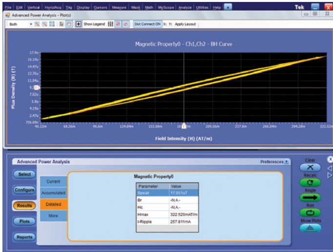
Figure 10. B-H plot for single-winding inductor as measured by the DPO7000 Series Oscilloscope and DPOPWR power analysis software.
