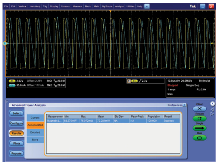
Figure 9. Power loss of a single-winding inductor as measured by the DPO7000 Series Oscilloscope and DPOPWR power analysis software.
