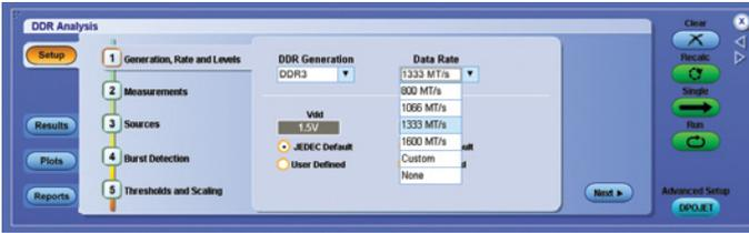
Figure 17a. DDR setup screen - Step 1.
