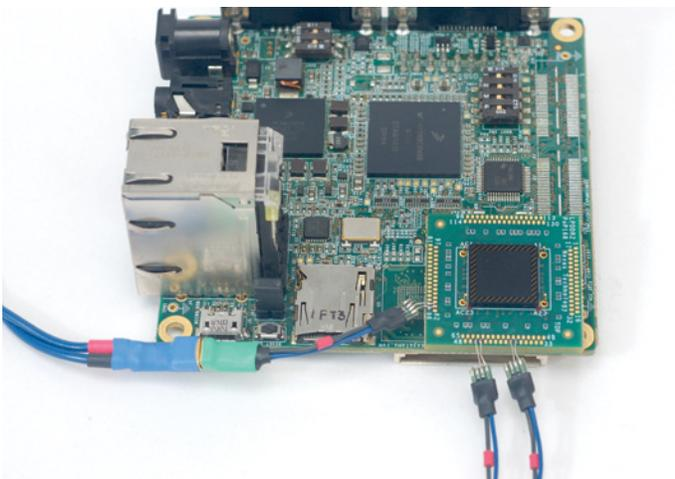
Figure 7. P7500 probe connected to LPDDR2 using PoP Interposer.
