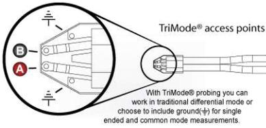
Figure 4. P7500 TriMode tip connections.
