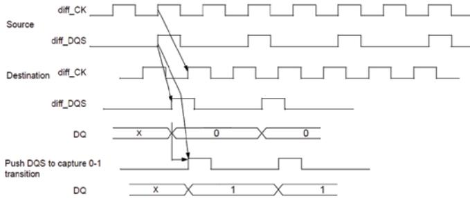
**Figure 21.** DDR3 Write leveling to deskew DQS and CK lines (source: JEDEC DDR3 SDRAM Standard, JESD79-3C ).
