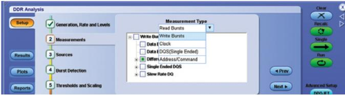
Figure 18. DDRA setup screen - Step 2 (measurement selection).
