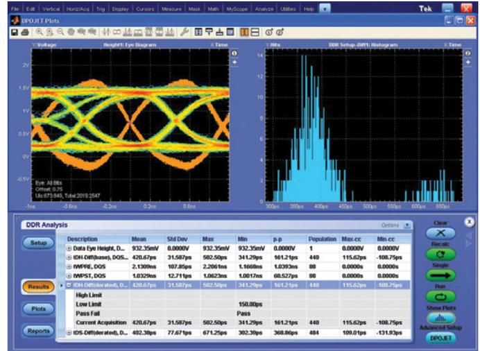
Figure 19. DDRA “Results” Screen showing two of the available plots.
