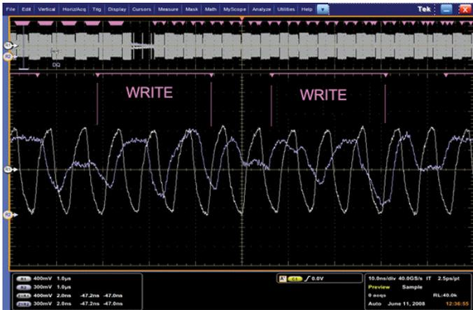
Figure 20. Back-to-back DDR3 Write operations.
