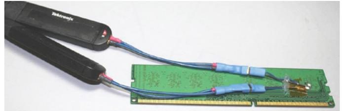
Figure 2. P7500 Micro-Coax probe tips soldered to DIMM.
