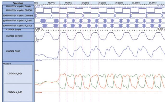
Figure 25. Using iCapture with a TLA7000 Series for System State views of a DDR design.
