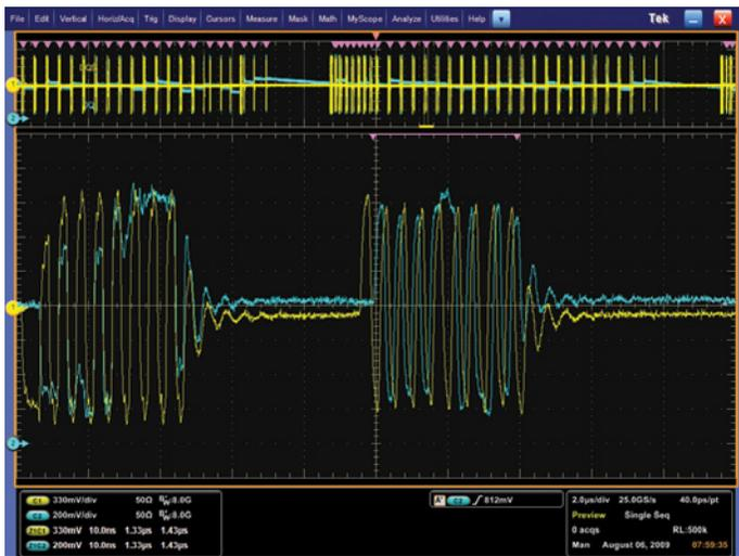
Figure 11. Using Advanced Search & Mark to identify all write bursts.
