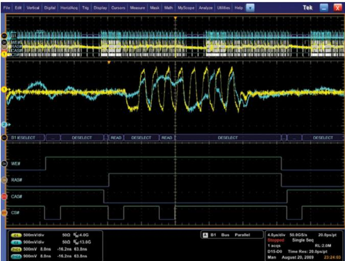
Figure 14. DDR3 Command Bus decoding on MSO70000.
