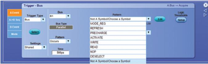
Figure 13. MSO70000 Symbol Trigger menu with DDR commands.
