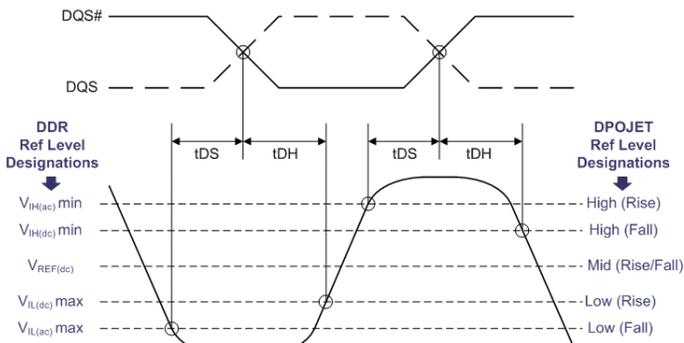
Figure 15. Measurement reference levels.
