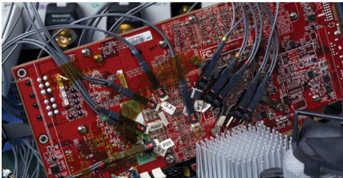
Figure 6. P6780 digital probe tips soldered onto GDDR5 PCB.
