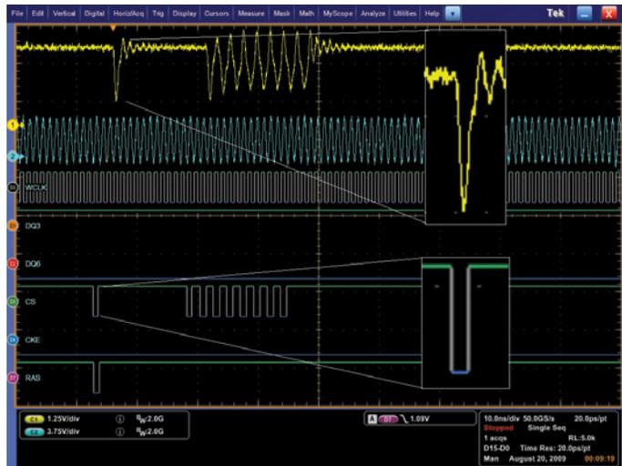
Figure 24. iCapture showing Chip Select line with analog and digital views.
