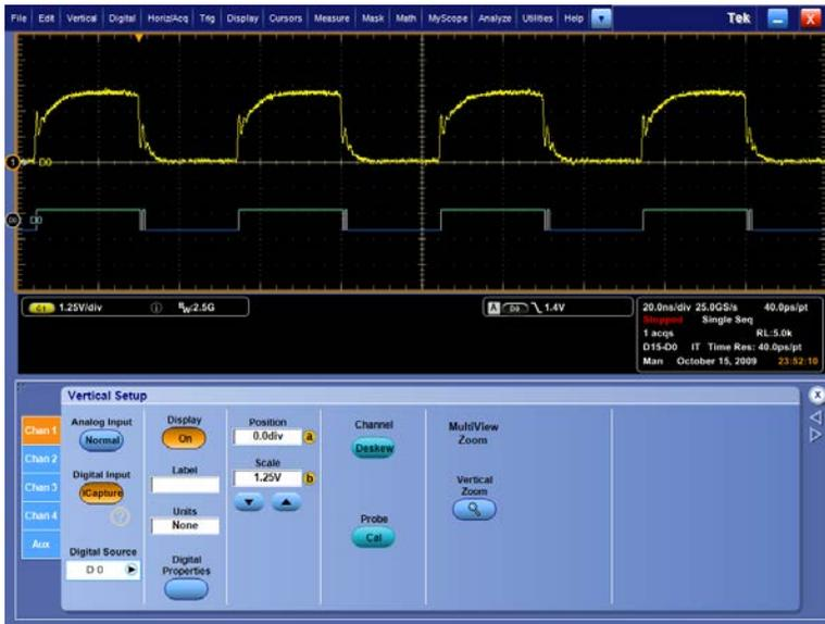
Figure 6. Edge ringing causing digital transitions.
