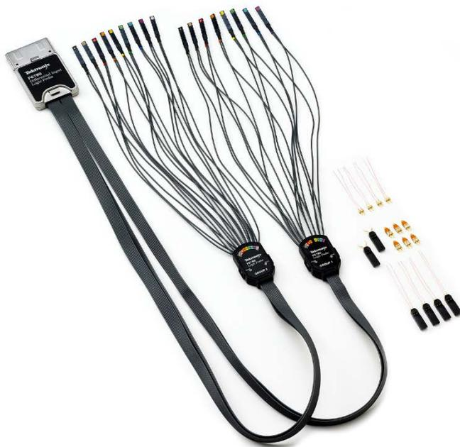
The probe inputs are 100 mil pin header compatible and the included accessory kit offer a wide selection of adapters including solder down probe tips providing connection flexibility. The P6780 Digital Logic Probe and iCapture Analog MUX gives you functionality similar to having 16 differential analog probes connected to the scope at the same time for a price similar to that of a single differential analog probe.
