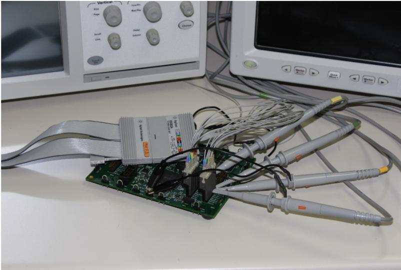
Figure 3. Substandard double-probing.
