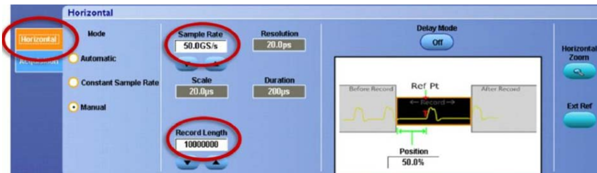
Figure 44: Set Record Length and Sample Rate
