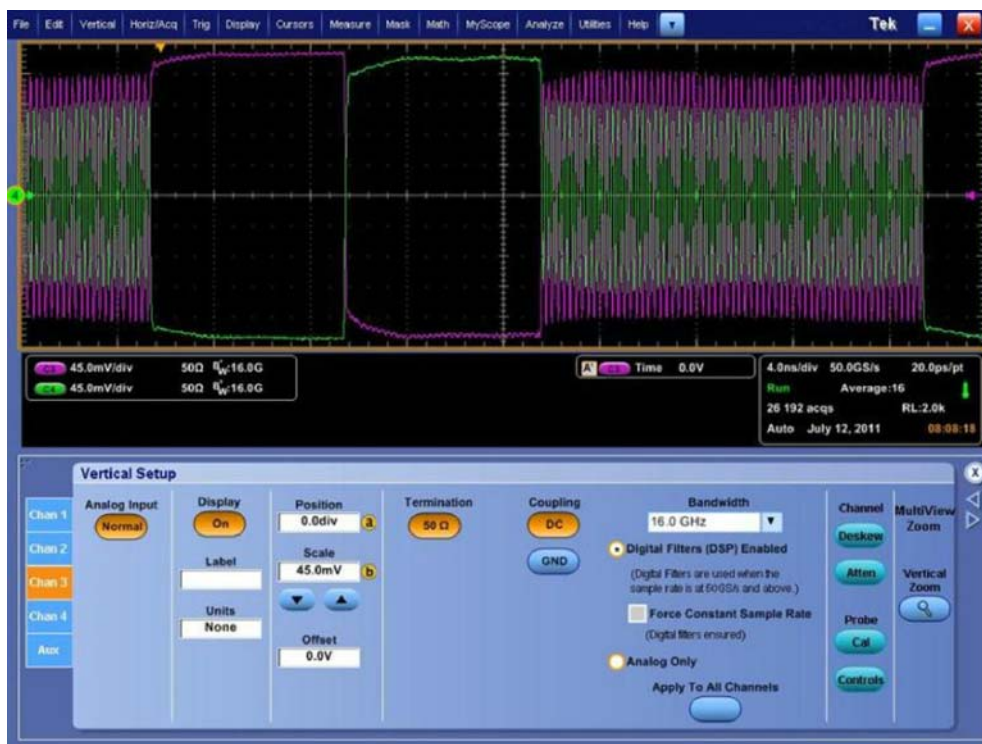
Figure 28: Vertical Setup Menu Displaying Example Configuration
