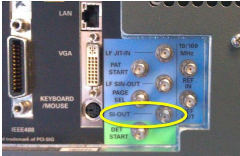
Figure 22: BERTScope Rear Panel with SI-Out highlighted. SI-Out should be connected to SI Input on Combiner. The BERTScope SI-Out will generate a 2.1GHz sine wave needed for Differential Mode Interference.
