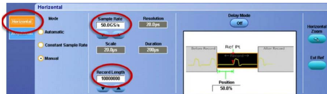
Figure 36: Set Record Length and Sample Rate
