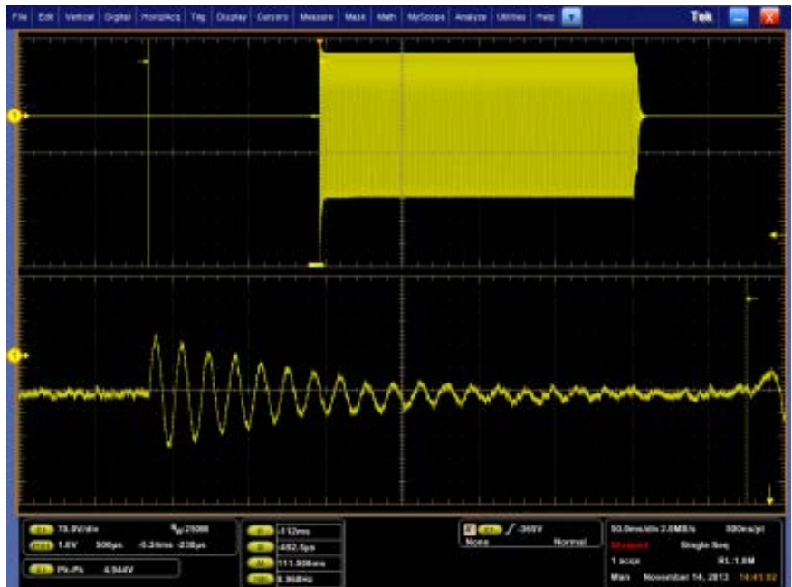
Figure 3. HiRes capture with >13 bits at 2 MS/s.
