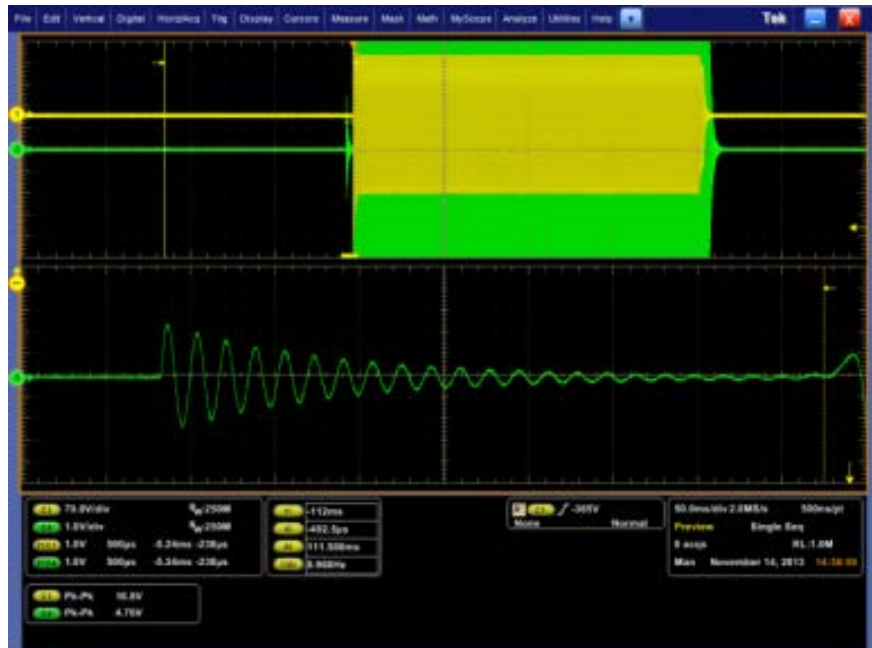
Figure 2. Dual channel capture with 8-bit resolution.
