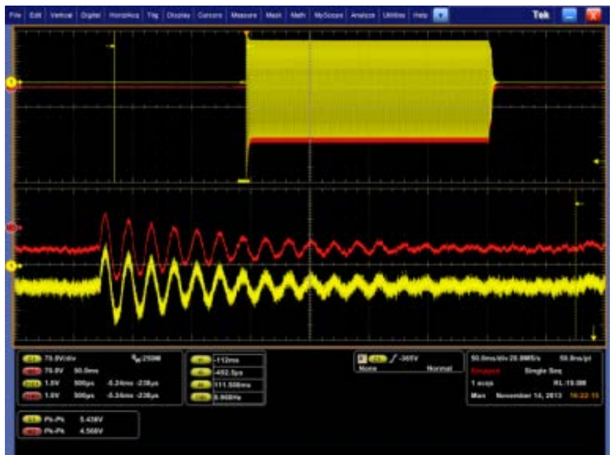
Figure 4. HiRes acquisition at 20 MS/s and low pass filtering.
