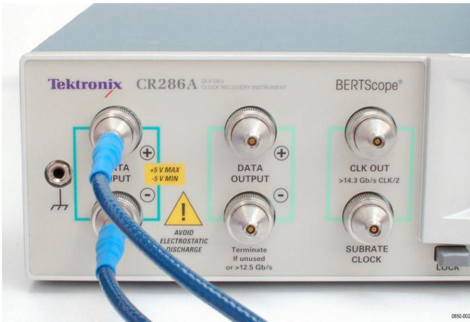
**Figure 7. CR286A front panel connections**
