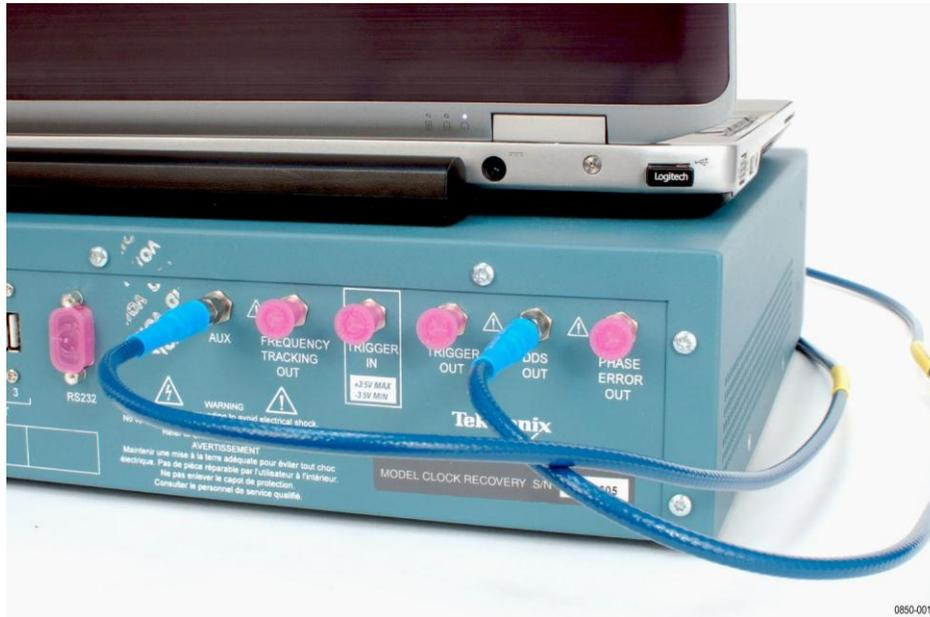
Figure 5. Clock recovery instrument rear panel connections
