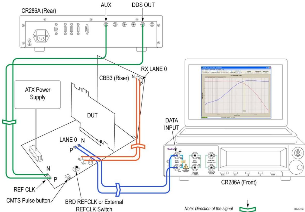
**Figure 4. Hardware connections from the clock recovery instrument to the CBB3.0 main board**
