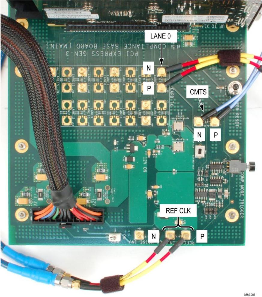
Figure 6. CBB3 fixture connector locations
