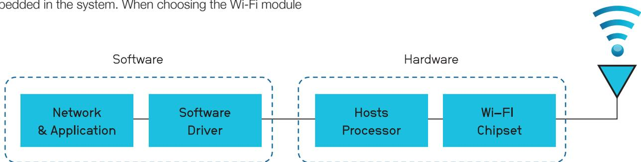
Figure 2. Simplified Block Diagram of a Typical Wi-Fi Module
