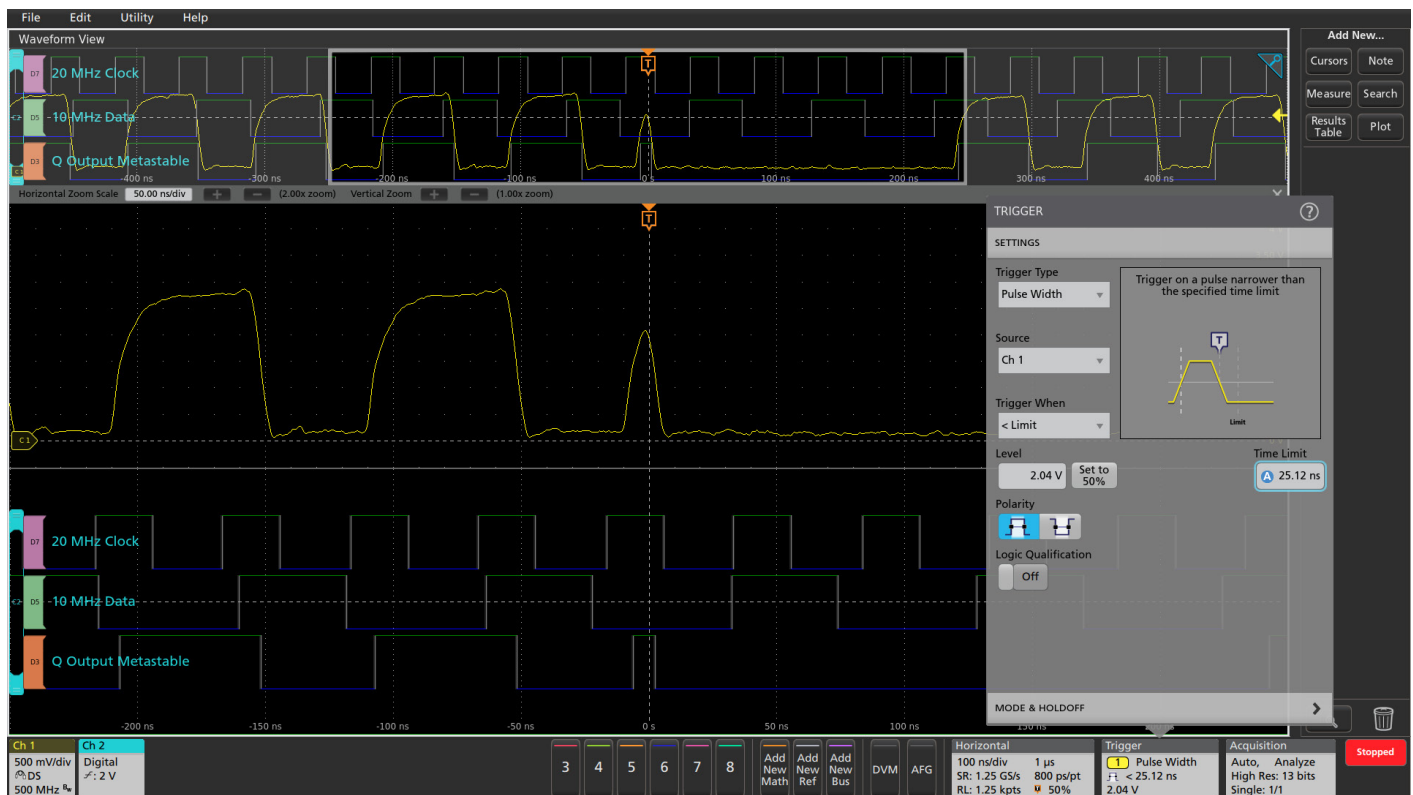
FIGURE 11. Pulse Width triggering captures a narrow glitch on the output of a 74LS74 flip-flop.
