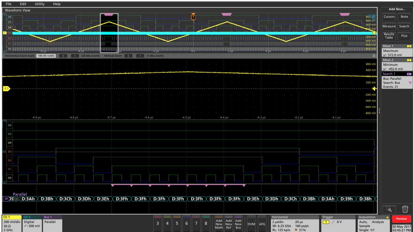
Reconfiguring the Wave Inspector Search and Mark for the maximum ADC output value of 3F yields 21 results. This should throw up warning flags, as there should only be three 3F values, one for each test signal peak. Looking at the zoom overview, the marks for the 3F values are grouped in three bunches over each test ramp peak. The zoom view over the decoded parallel bus values shows the expected progression of values 3A, 3B, 3C, 3D, 3E, up to 3F where instead of a single value there are seven.
