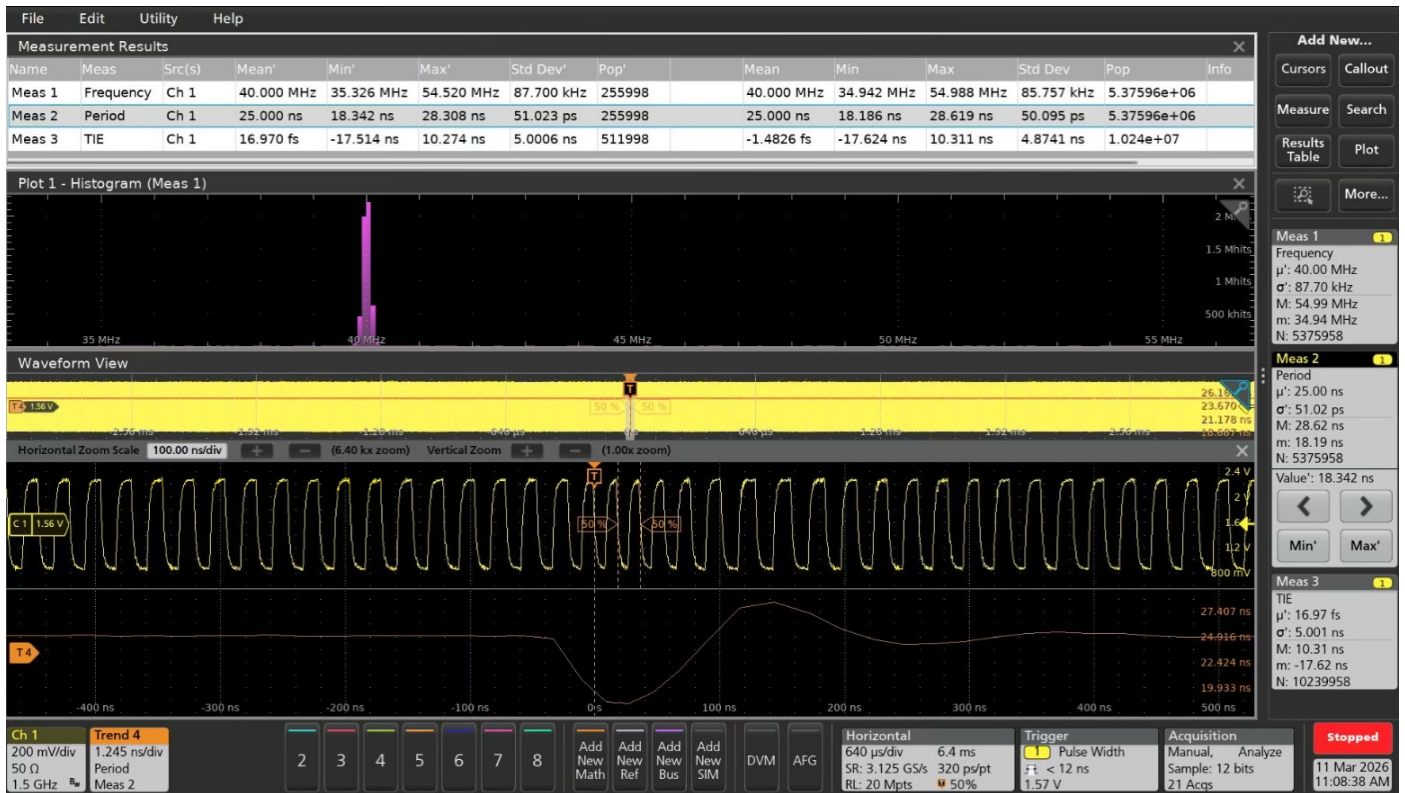
Figure 1. Frequency, Period and TIE results of a 40 MHz clock. Note the few cycles where the periods get shorter than expected on T4 trace.
