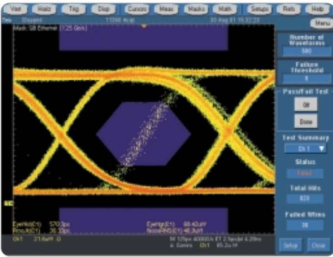
► **Figure 2.** A gigabit ethernet eye diagram being tested for pass or fail.
