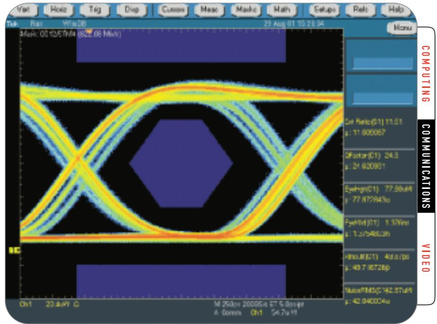
► **Physical layer testing of electrical and optical telecom and datacom signals up to 2.5 Gb/s.**
