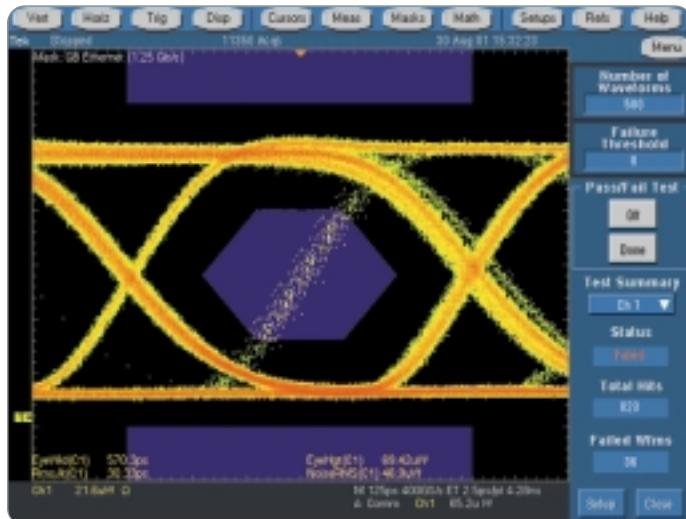
► Figure 2. A gigabit ethernet eye diagram being tested for pass or fail.
