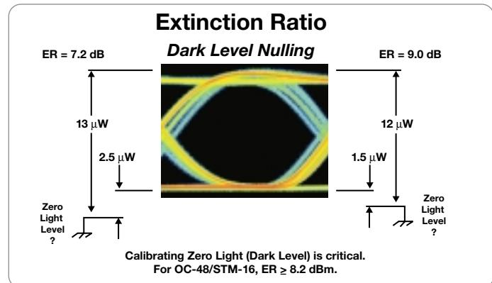
► **Figure 7.** A zero light level change can affect the extinction ratio value.
