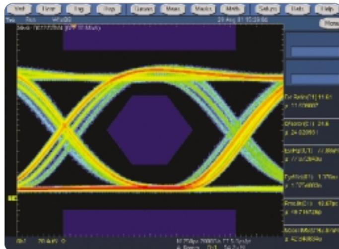
► **Figure 10.** Intensity-graded eye crossing display.
