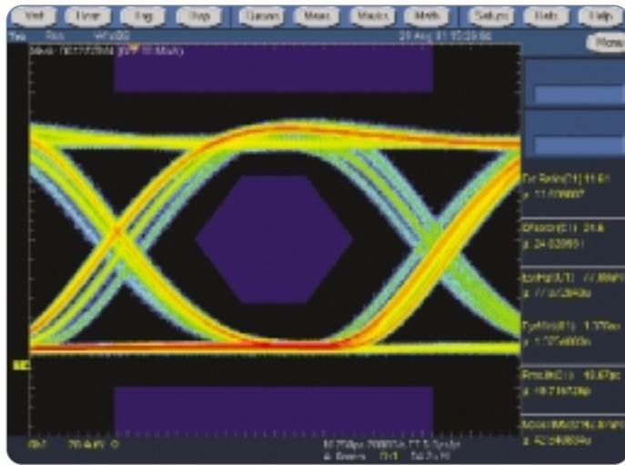
► **Figure 10.** Intensity-graded eye crossing display.
