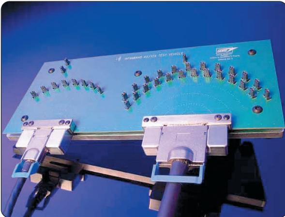
► **Figure 1.** InfiniBand-to-SMA breakouts allow you to connect the 50-Ohm signal paths directly into the 50-Ohm inputs of the oscilloscope.
