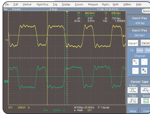
► Figure 4. Quickly checking rising edge-to-rising edge timing between two signals is easy with the screen-based cursors.
