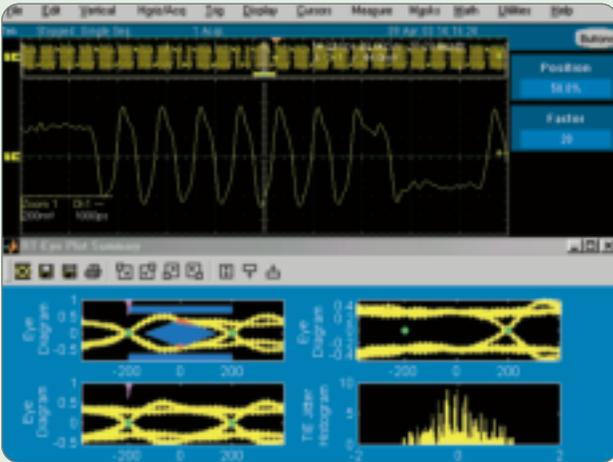
► **Figure 7.** A high-performance, real-time oscilloscope, paired with RT-Eye™ software, provides a turnkey solution for serial data validation and compliance.
