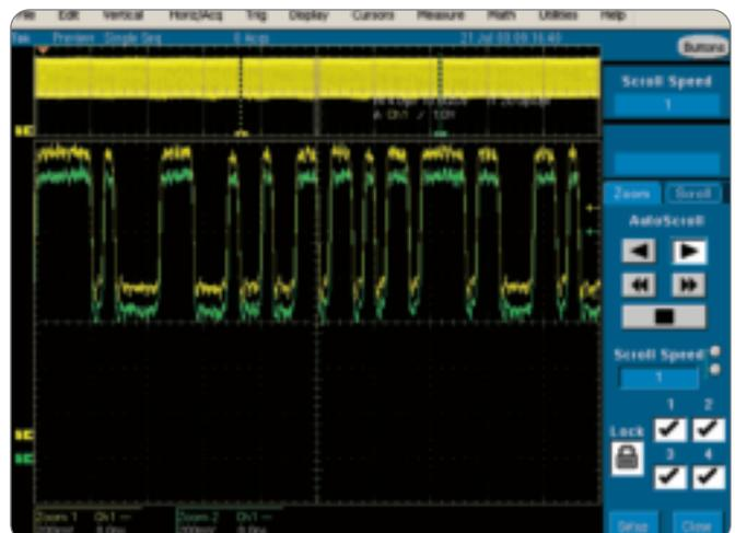
► **Figure 10.** Two locked zoom regions being automatically scrolled.
