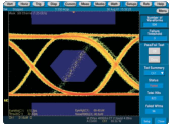
► Figure 5. Eye diagram showing faulty bit.
